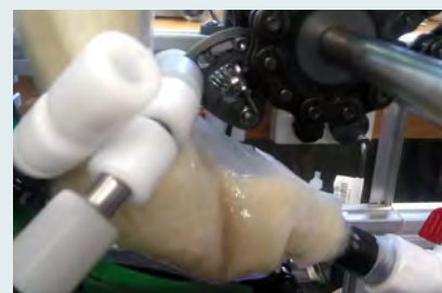
Mechanical rollers manipulate the soft-walled 'stomach' to digest couscous.
